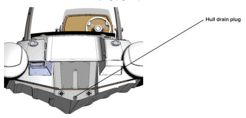
Fig. 28. The hull drain plug is located on the transom.
