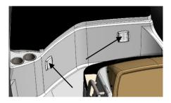
Fig. 1. Ventilation openings on the bow locker.
