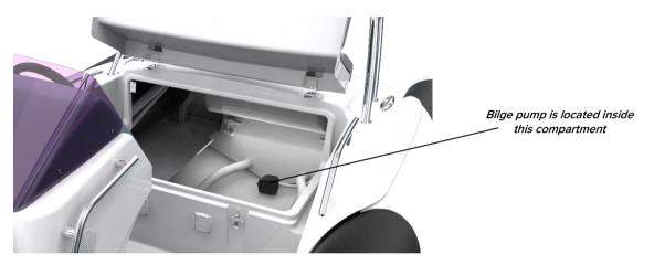
Fig. 25. Interior space of rear ccompartment with bilge pump inside of additional section.
