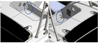
Fig.30 Bow lifting eyes, 2 positions.
