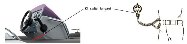
Fig. 20. Engine kill switch lanyard.
