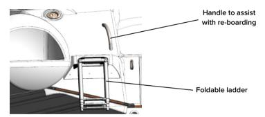
Fig. 5. Foldable ladder and handle for assistance with re-boarding.
