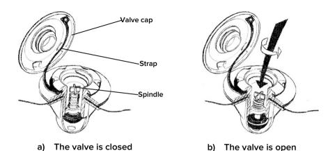
Fig.9. Design of the inflation valve (option 1).
