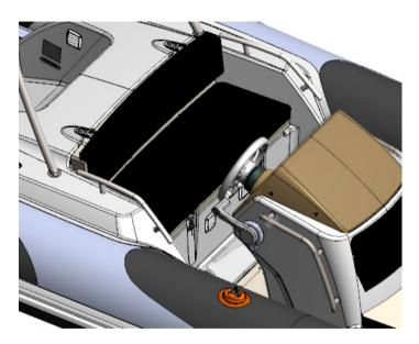
Fig. 33. Rear locker with access panel, lifters, soft seat and seat back.
